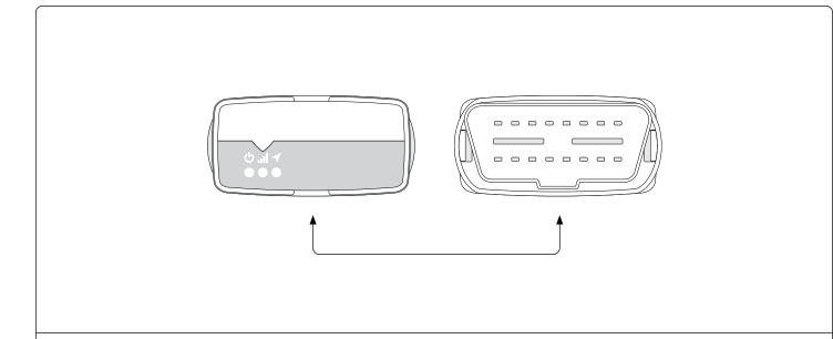
**Step 6:** Ensure the GPS antenna (located at the "bottom" of the GO device) is facing away from any metal surface. See diagram above.
